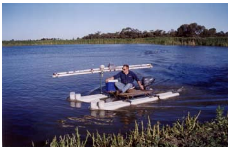
Channel leakage surveys
